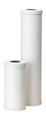
Pentair<sup>‡</sup> Pentek<sup>‡</sup> RFC Series Cartridges are constructed with a 70-micron porous polyethylene outer shell and durable polypropylene endcaps. The 2-3/4" outer diameter cartridges have a polypropylene core and the 4-1/2" outer diameter cartridges incorporate a spun polypropylene core. Sandwiched between the outer shell and the core is a bed of granular activated carbon (GAC).
