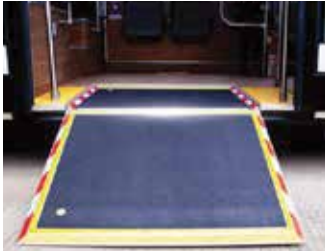
Flip ramp for wheelchair access
