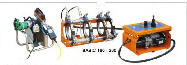
**BASIC 160/200** is able to weld fittings such as elbows, tees, Y-branches and flange necks without any additional equipment by simply fixing the clamps' drag bar.
