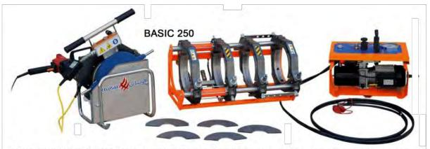
**BASIC 250/315** is able to weld fittings such as elbows, tees, Y-branches and flange necks without any additional equipment by simply fixing the clamps' drag bar.
