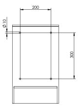
Dimensions of the collecting pan All dimensions in mm
