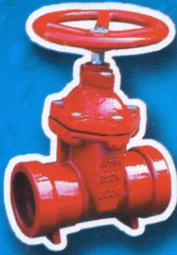
Push-on joint ends gate valve Non rising stem Ductile iron DN50~300 AWWA C509
