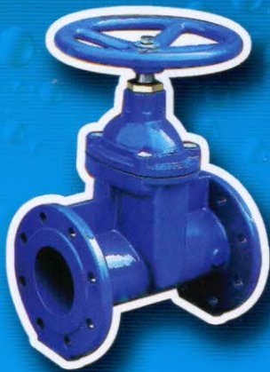
Flanged gate valve Non rising stem Ductile iron Soft sealing DN50~600 PN10-16
