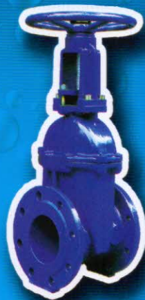
Flanged gate valve Rising stem Ductile iron Soft sealing DN50~600 PN10-16
