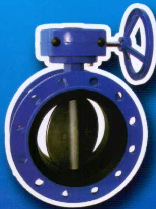
Flanged butterfly valve with gear box Ductile iron Soft sealing DN50~2200 PN10-16
