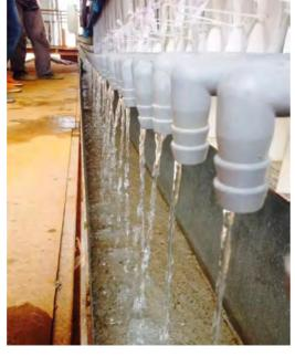
Filtrate that passes through filtration cloth is collected through collection pipe.
