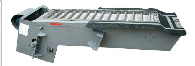
This automatic bar screen is mainly composed of electric motor, gearbox, steel frame, tooth rake, and transmission system. Electric motor and gearbox are mounted at the head of steel frame, together with driving sprocket and traction chains, forming the driving system.
