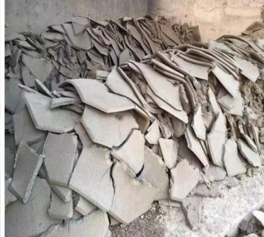
The slurry is fed to filtration chambers and the sludge cakes are accumulated. As the sludge cake becomes thicker, the filter resistance increases as well. When the separation chambers are full, the filtration process is stopped as the optimum pressure difference is reached.
