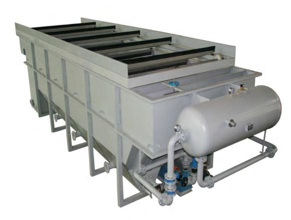
The feed water to DAF float tank is often (but not always) dosed with a coagulant (such as ferric chloride or aluminum sulfate) to coagulate the colloidal particles and/or flocculants to conglomerate the particles into bigger clusters.
